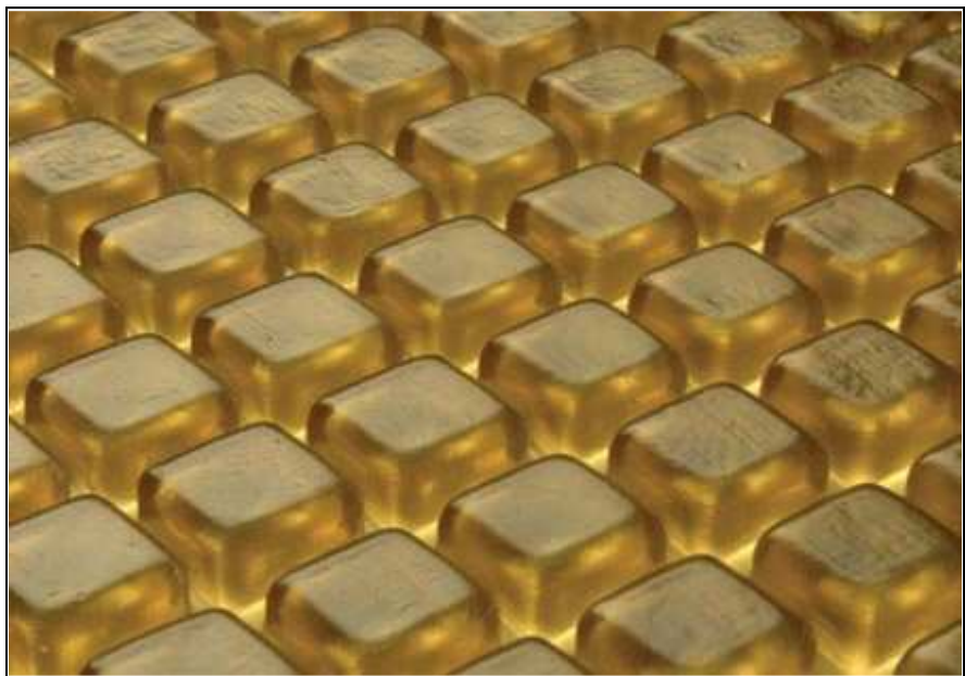
Akton viscoelastic polymer, manufactured by Action Products, provides pressure reduction properties, as well as shock absorption and vibration damping for medical applications.
